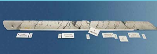
ABOVE: A cored hydraulic fracture from a Multiwell Experiment fracture created in 1983. Core was taken in 1988. The hydraulic fracture has many individual strands. Photo courtesy Norm Warpinski.
